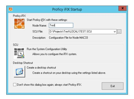
This screen is the default screen that starts up when iFix is installed. Using this we can configure all our projects. We will be able to configure them to launch directly after we have set them up.
